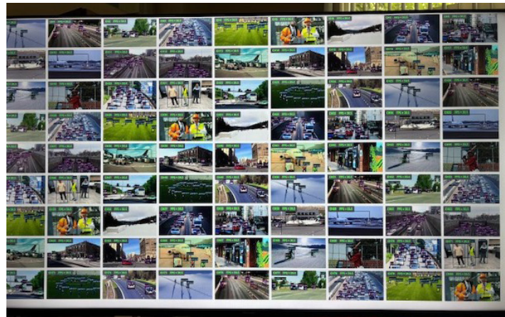
Figure 1: 81 decoded HD video streams on a YoloV5s model 320x320 resolution. Each video with 30 fps inference per video stream. Models run on four MemryX M.2 modules on a PCIe carrier card with less than 40W total AI accelerator power consumption. AMD x86 Ryzen processor used for demonstration.
